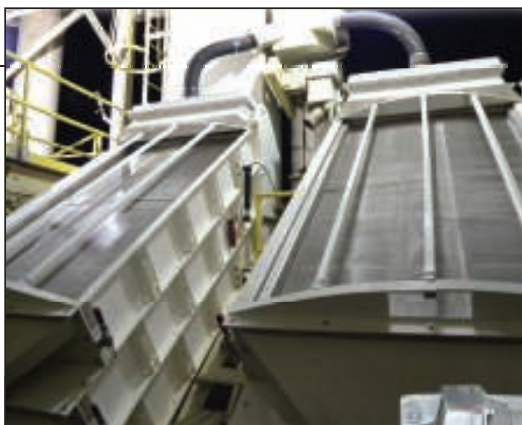
FIGURE 5. Unlike vibrating screens that shake the entire screen box, the Overstrom fine mesh screener vibrates only the screen cloth, which offers many benefits
