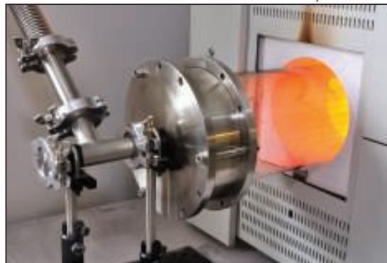
FIGURE 5. The CVD furnace used in Graphene Frontiers' production process is operated at atmospheric pressure
