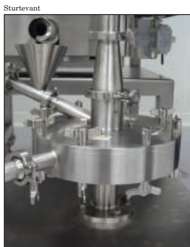
FIGURE 2. The Micronizer jet mill can process chemicals to nanometer scale while providing a tight particle-size distribution
